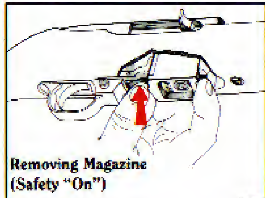
Figure 3. The safety should be “on” when the magazine is being removed or inserted. When the forward section of the magazine latch is pushed in (pivoted upward), the magazine is released. Depress the latch with the thumb and at the same time grasp the magazine between the thumb and forefinger and draw it out of the gun.
